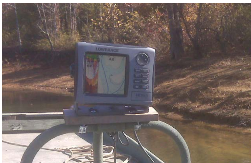
Sonar unit used in Kerr Lake Surveys
